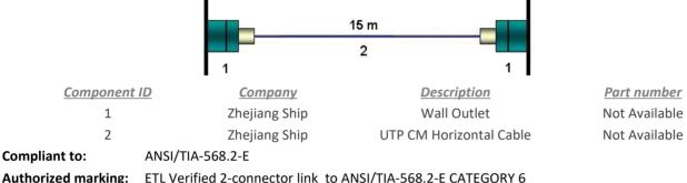
ETL Verified 2-connector link to ANSI/TIA-568.2-E CATEGORY 6 Must include channel illustration and part numbers
